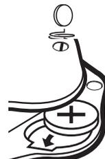
**Important:** While replacing the backup battery, the 3 “AAA” batteries must be kept in Vapor or Vapor must be connected to the AC adaptor while the adaptor is plugged in. If not, you will lose all saved information.
